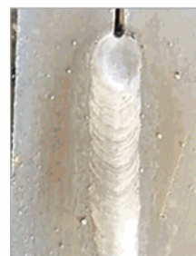
Joint 8mm steel plate with φ3.2 electrode
