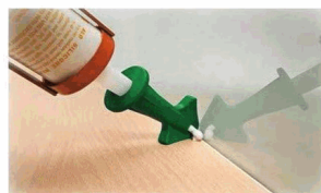
Pushing silicone caulking gun smoothly
