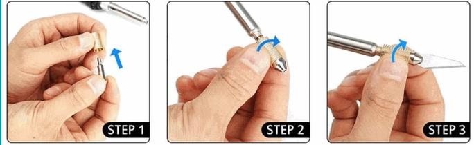
· Screw the hot knife chuck, insert the blade to the chuck, then tighten the screw ·
