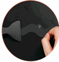
Exhaust the air with scraper
