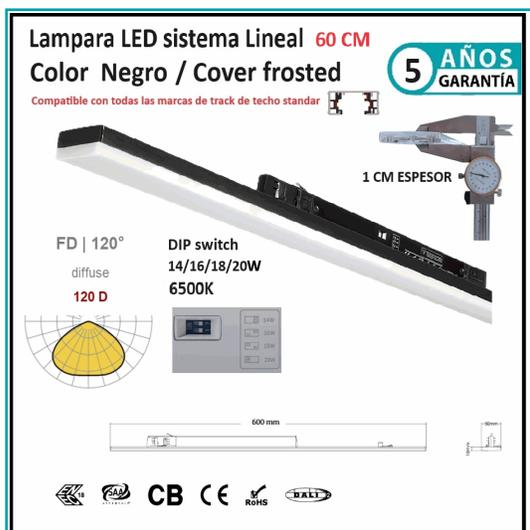
Lampara 6500K Lineal 60 Cm Negra Frosted 3200Lm 20W Dip Ajustable 14/16/18/20W Cri90 3 Cables Ac100-227V
