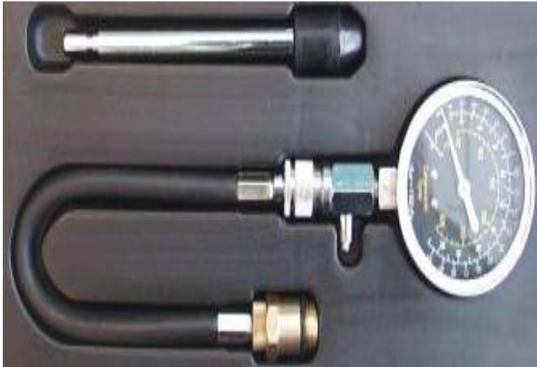
Tool name: Cylinder pressure gauge Function: Check the cylinder pressure.
