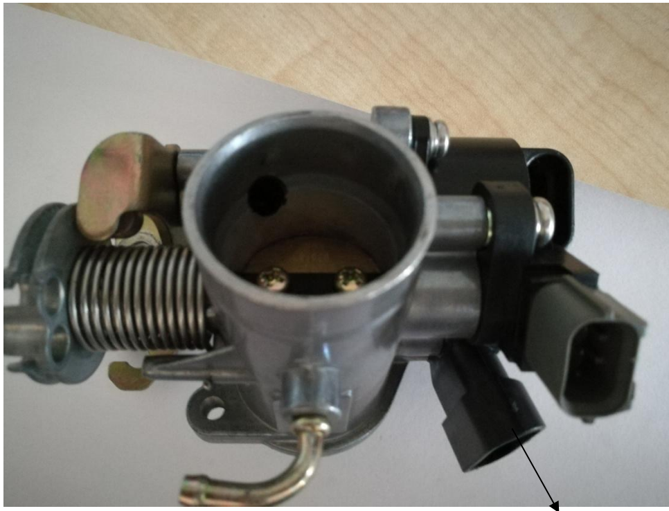
Intake pressure sensor / intake temperature sensor (integrated)
