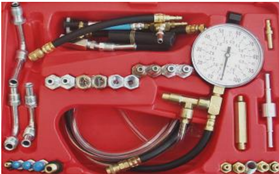
Tool name: Fuel pressure gauge Function: Check the fuel system pressure, and judge the working conditions of fuel pump and fuel pressure regulator in the fuel system.
