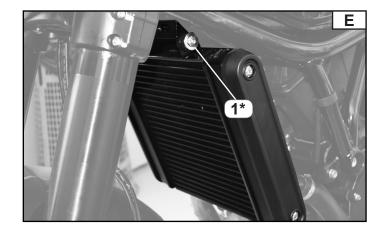
The screws (1\*) fastening the lower bracket to the frame Fig. F.
