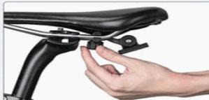
2. Rotate the buckles to fix.
